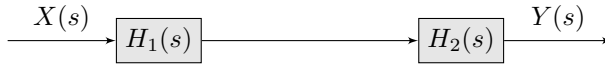
Figure 8: Transformation of input and output to Laplace domain for a series connection.
